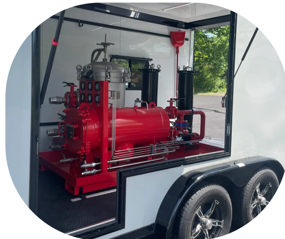
Mobile Fuel Polishing & Tank Cleaning System Ready For Deployment
